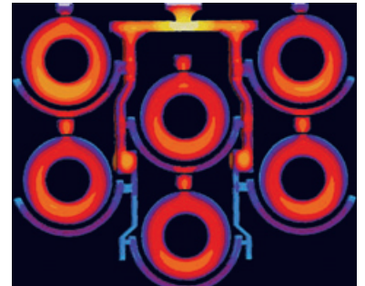
MAGMA – solidification of a break disc pattern
