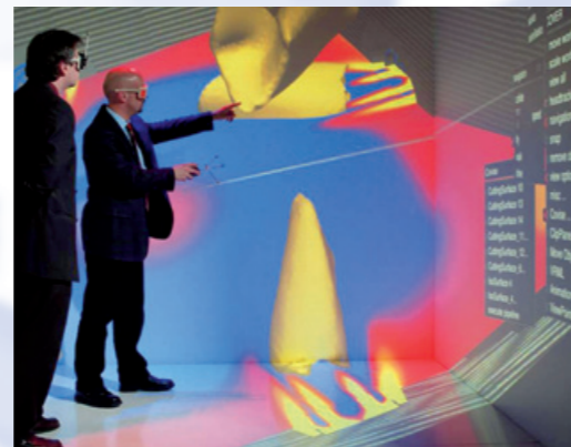
Computer-aided analysis of flame interactions in a 300 MWe combustion chamber in the Virtual Reality
