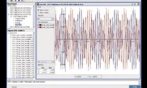
ROBOTIKER · IQ signals directly captured from FPGA by logic analyzer
