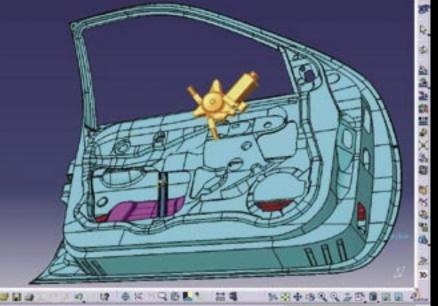
CEA-LIST - study of accessibility: assembly of a control device of car door windows
