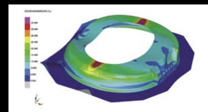
GNS - deep drawing simulation of a wheel arch
