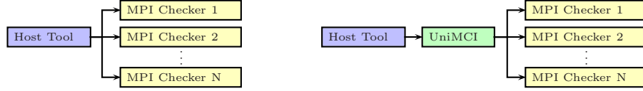
(a) Integrations without UniMCI (b) Integrations with UniMCI Figure 1. Integrating a host tool with correctness checking tools.
