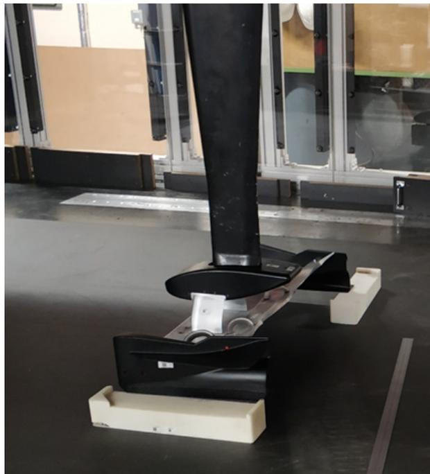
Figure 21: Imperial Front Wing assembly on Imperial College London 10x5 Wind Tunnel.
