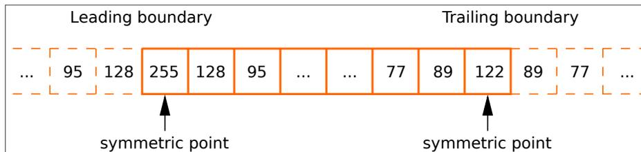
Figure 28: Symmetric extension at the leading and trailing boundaries of a signal segment.
