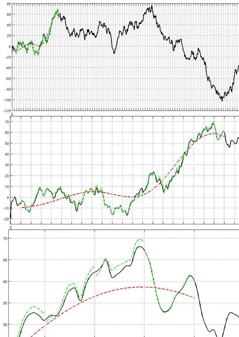
Figure 44:  $n_c = 10$  checksums have been created for the black line data stored on  $n = 100$  nodes. The data for  $n_l = 20$  nodes is removed. Exact recovery from the checkpoint is not possible, but incomplete information recovery by solving the optimization problem with constraint 111 and approximate data as indicated by the red line. The output from the solution procedure is marked in green. (a) full view. (b-c) zoomed in.
