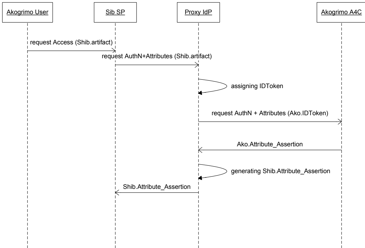
Figure 31 Message Flow for Akogrimo user accessing a Shibboleth resource with focus on attribute transmission. The bridging element acts as Shibboleth Identity Provider and Attribute Authority.
